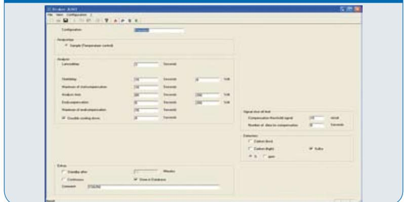
Program settings allow you to select all necessary conditions, such as parameters for HF furnace power and time for one specific application; these can then be stored as a set of configuration under a free selectable name. It is easy to call up different configurations for each application.
