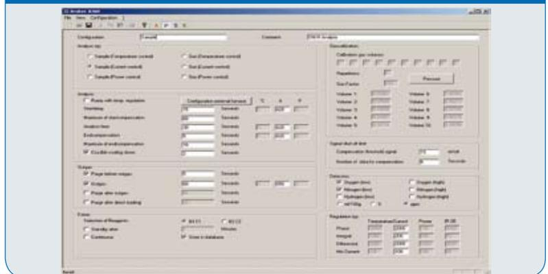
Program settings allows you to select all necessary conditions, such as parameters for temperature and time for one specific application; these can then be stored as set configuration under a free selectable name. It is easy to call up different configurations for each application.
