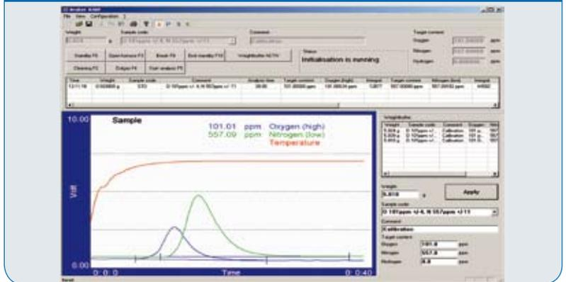
You can perform all analyses and signal performance tasks on the Analysis screen. Current signal data will be presented graphically. The results of the last five analyses are shown simultaneously. Even at later times you can call up any information in the result manager on this screen.
